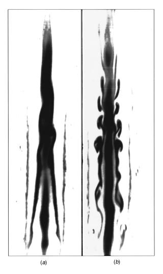
Fig. 12 LIF photographs showing an upward traveling vortex breakdown, for a case with  $D/\sigma_0=4.3$  and S/D=1. The flow is illuminated in a vertical plane, where the bottom of the plane is 27 cm above the sphere center. In (*a*), the leading part of the breakdown is observed to have the form of a kink in the vortex, which is followed in (*b*) by organized turbulent structures wrapped around the inner part of the vortex core.
