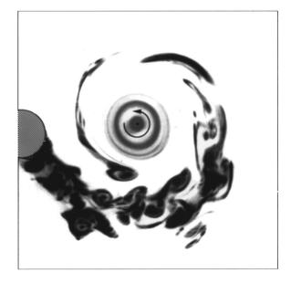
Fig. 5 LIF photograph in the horizontal plane *B* showing the sphere wake entrainment into the primary vortex core for a case with  $D/\sigma_0=4.3$  and S/D=2
